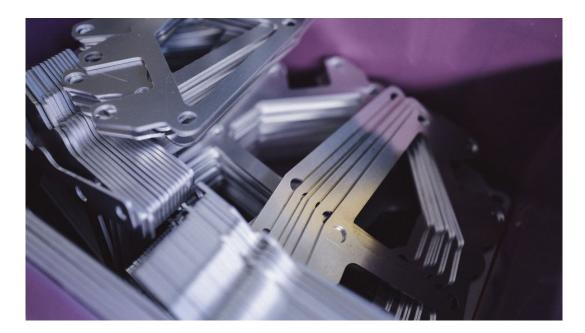
Useful feature: the ejector cylinder mounted on the cutting head helps the machine release smaller sheet metal parts from the scrap skeleton. Finished parts are intercepted by a retractable sorting flap, and the SortMaster Box Linear distributes them into up to eight containers beneath the machine.
