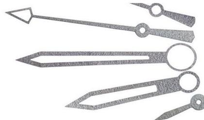
Cutting to specification with an ultrashort pulse laser: watch hands made of 0.05 millimeter thick stainless steel. The slotted recesses provide space for a subsequent application of fluorescent material. Picture: TRUMPF
