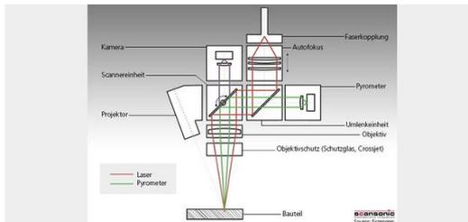
The coaxial arrangement of the pyrometer with respect to the laser beam enables precise temperature measurement.
