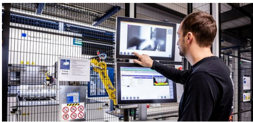
<p class="MAGAFIetext">The TecZone Bend programming software in combination with SimulEasy ensures process reliability. This allows 3D simulations including collision monitoring to be generated before the bending process.</p>
