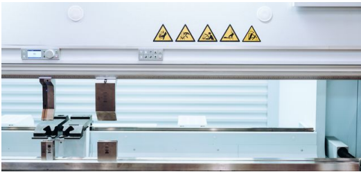
BendGuard is a safety system for TRUMPF machines, ensuring the safety of the operator.
