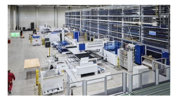
The wide product range demands the highest possible flexibility from the Competence Factory. In the approximately 8,200 square meters of the production hall, this is helped by a 50-meter Stopa store that is connected to punching and bending machines and feeds them the material.
