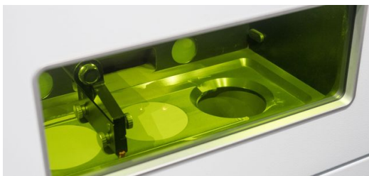
Process data such as the laser melt pool and powder application are monitored independently by the TRUMPF systems. (Source: TRUMPF)
