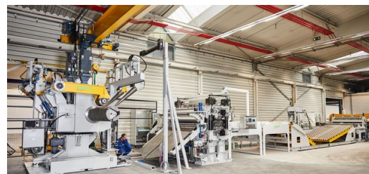
As well as the TRUMPF VarioPress 500, Wagner has also invested in a new decoiling system. Picture: Florian Bilger
