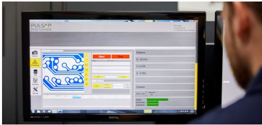
The Photonic Elements machine control software displays the ablation geometry executed during the process. (Picture: Claus Langer)
