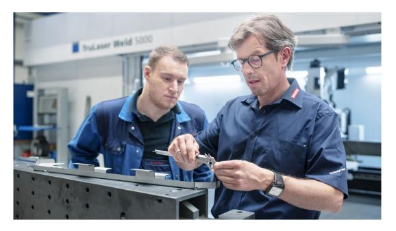
Deep penetration welding with a laser involves far less heat input than conventional welding methods – and that means less distortion. Josef Böhmer (right): "Parts nowadays have to be made to such fine tolerances, especially in formwork construction. So we save a lot of time by not having to straighten them after welding! © Günther Bayerl
