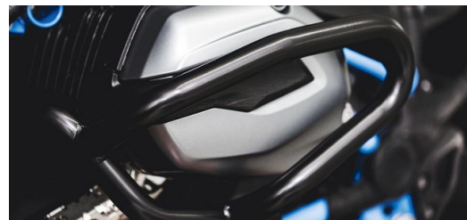
IBEX aims to make everything people need for their motorcycles out of sheet metal. These crash bars are just one example of what the company offers.
