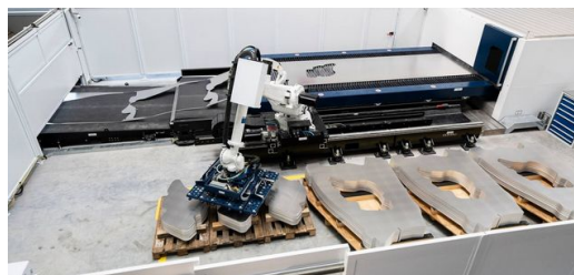
Laser blanking: A robot automatically sorts the cut components.
