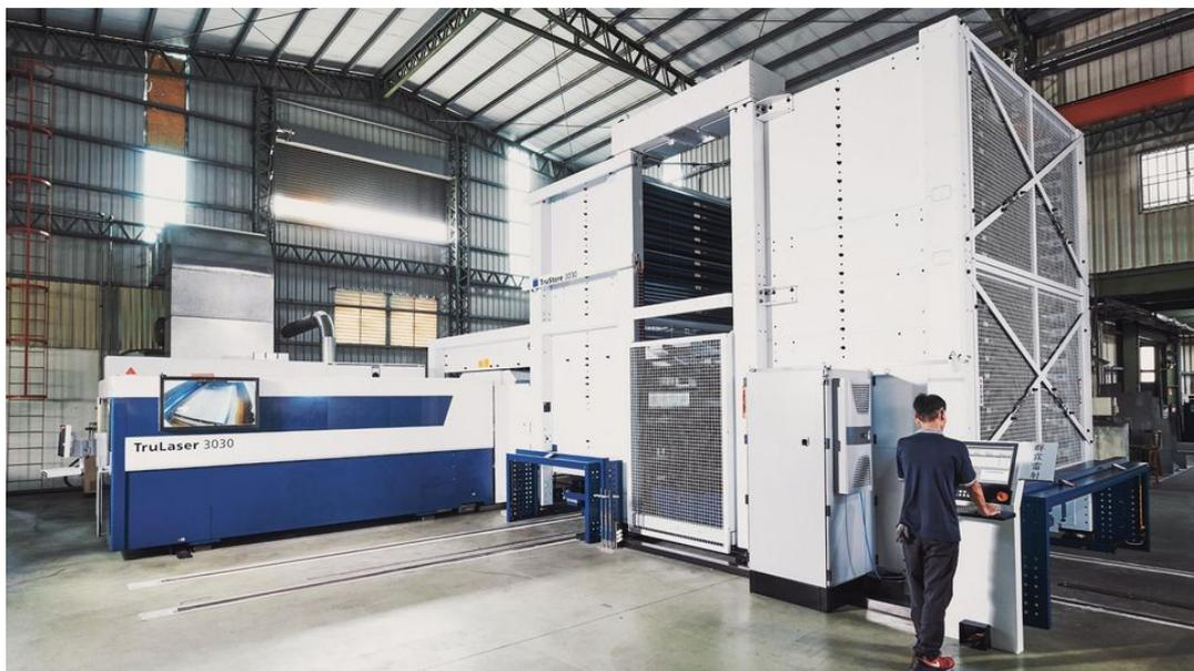
As an introduction to automated production, CHUN-LIN decided on a TruLaser 3030 fiber with connection to a TruLaser 3030 universal storage system. The connected universal storage system has two storage towers with 31 pallets for large sheets with maximum dimensions of 3,000 x 1,500 millimeters.
