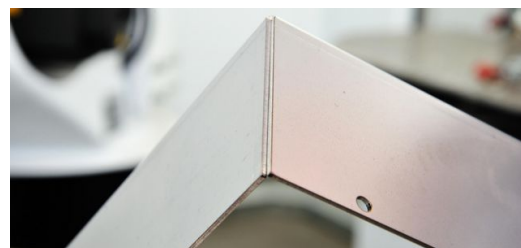
"Tolerant" laser welding is essential for components that have gaps or awkward overlaps. The TruLaser Weld 5000 offers this capability with its optional FusionLine feature. Image: Peter Klingauf
