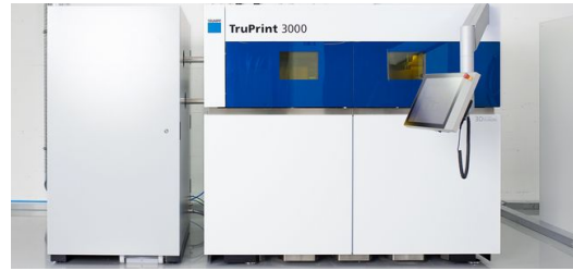
-The 3D printer - here the TruPrint 3000 from TRUMPF, prints the component layer by layer. (© Clauss Morgenstern)
