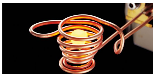
A coil envelops a fusion crucible. The material to be melted is put into the crucible and heated. Alternating current flowing through the coil, generates an electromagnetic field which transfers the electrical energy to the melting stock in a non-contact manner. (Image: TRUMPF)
