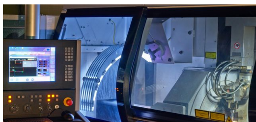
With the TruLaser Tube 7000 the tube specialists of ProfilaseRichter have opportunities that many customers don't even know, yet. Examples are bending connections and also positioning aids with locating pins and cut-outs to simplify assembly. Thanks to the degree of automation in the machine the throughput times are shorter and so are the delivery times. Picture: Escherich Fotografie
