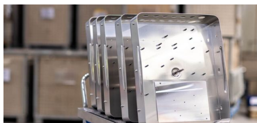
CoolCase manufactures housings for the inverters of solar systems.
