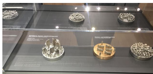
Substrate plates with 3D-printed dental prosthesis.
