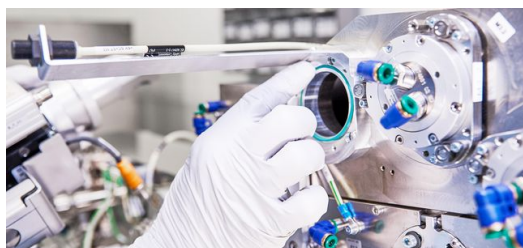
A mechatronics engineer installs a mirror mounting.
