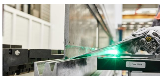
The backgauge system of the new TRUMPF EHT VarioPress 500 is coupled with CNC-controlled bending aids and a clamping device. Picture: Florian Bilger
