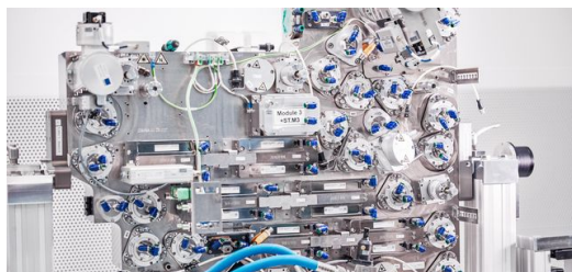
Mirror support on a EUV-module
