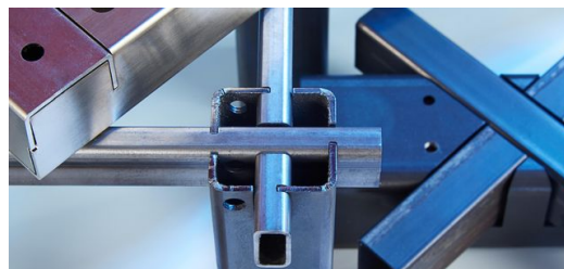
The TruLaser Tube 7000 cuts tubes and profiles with outer circle diameters of up to 254 millimeter. Complex calculations at corners of rectangular profiles are automatically handled by the TruTops Tube software. Picture: Escherich Fotografie
