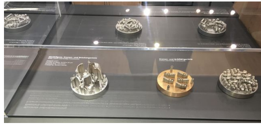
Substrate plates with 3D-printed dental prosthesis.
