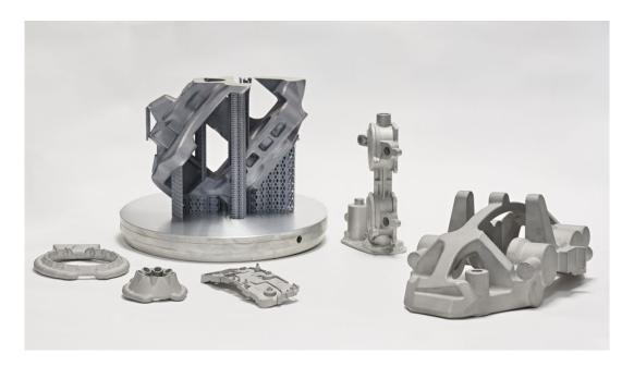
The ADaM team now uses TRUMPF 3D printers for a whole range of parts, including mirror units, brake calipers and housings for control units and displays.
