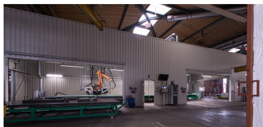
Photon AG manufactures rail car side walls up to 25 meters long in its laser cabin. Picture: Angelika Grossmann
