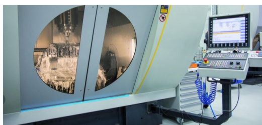
A Zeiss system grinds and polishes a mirror for EUV production.
