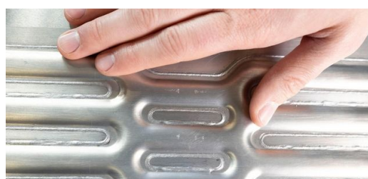
In the folding-box concept developed by BENTELER for a stainless steel battery housing, the patented TRUMPF solution BrightLine Weld ensures spatter-free processing and high-strength gas- and helium-tight weld seams, even in rapid series production.
