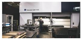
"At our company, non-productive times are sometimes longer than cutting times. That's what makes fast set-up so important," says Fabian Renz from Rieber. The advantage of the <a href="TruLaser Cell 7040">TruLaser Cell 7040</a>: It offers two flexible stations so that the operator can set up and manufacture at the same time.
