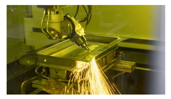
Deep drawing is one of the most important manufacturing processes at Rieber. But after that, a flexible tool is needed to precisely cut off the edges before joining the deep-drawn components. This is what the TruLaser Cell 7040 with an integrated TruDisk 3001 disk laser is for on the Rieber factory floor.
