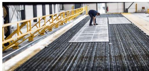
Because the table of the laser machine is at ground level inserting sheets is easy (Photos: Norbert Voskens).
