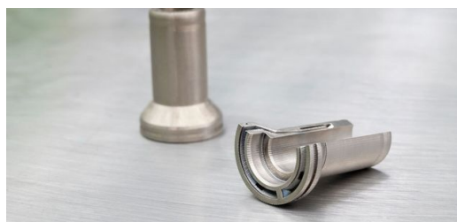
Amorphous metals are produced by flash-freezing molten metals. The atoms solidify in a random arrangement and do not form crystal structures.
