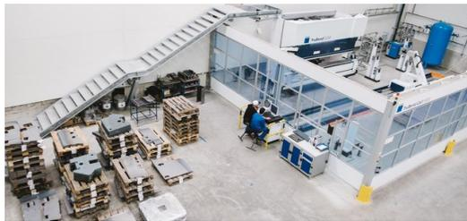
With its 230-tonne press force, the TruBend Cell 5000 can process components of 3000 x 1500 millimeters conveniently.
