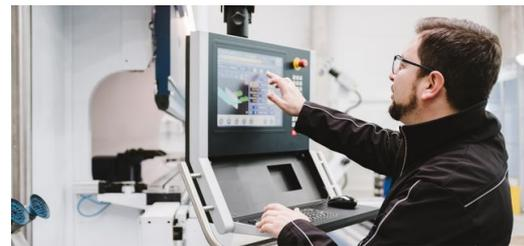
The TruBend Cell 5000 gives Martin Mitterhumer all of the options that are important for him, such as the camera-based, sensor-controlled position recognition and easy intuitive handling.
