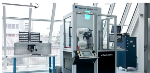
Efficient duo: At the Widnau site in Switzerland, endoscope manufacturer Karl Storz welds eyepieces on a TruLaser Station 7000. A mobile robotic cell takes care of loading and unloading the components.
