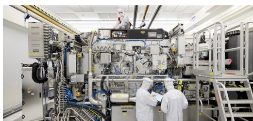
ASML employees working on a new generation of the EUV lithography system NXE3400B.
