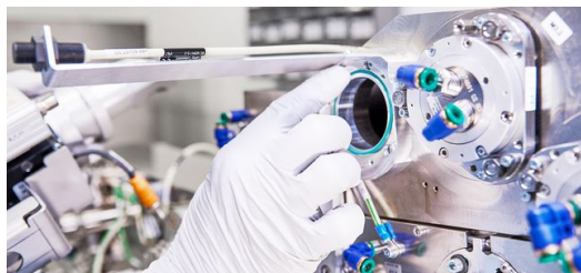
A mechatronics engineer installs a mirror mounting.
