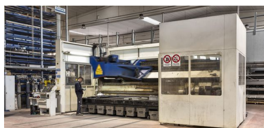
Multi-talented: ELFIM does not just use the Lasercell 1005 to weld and cut 2D and 3D components. The system is also suitable for laser metal deposition.
