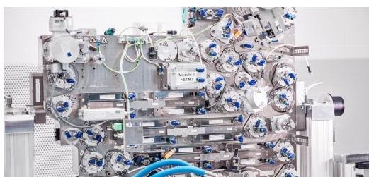
Mirror support on a EUV-module
