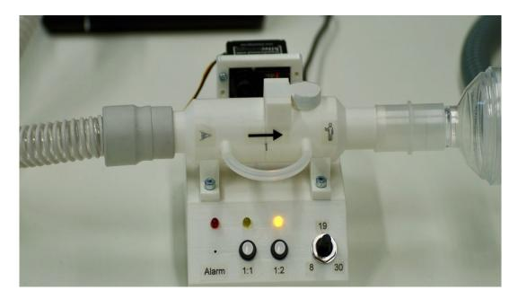
With the help of 3D printing, researchers from "The Breathing Project" have developed a device for converting an anti-snoring device into a ventilator. This is to be used in caring for coronavirus patients. (Source: University of Marburg)
