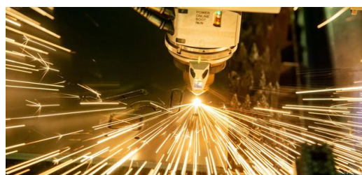
With EdgeLine Bevel technology, a TRUMPF standard machine for laser cutting produces beveled cutting edges on the contours of the component.
