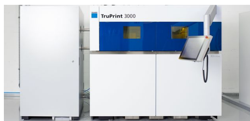
-The 3D printer - here the TruPrint 3000 from TRUMPF, prints the component layer by layer. (© Clauss Morgenstern)
