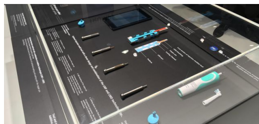
Who would have thought? 3D printing also changes toothbrushes - at least in their production. The new tool for the plastic attachment has been produced additively.
