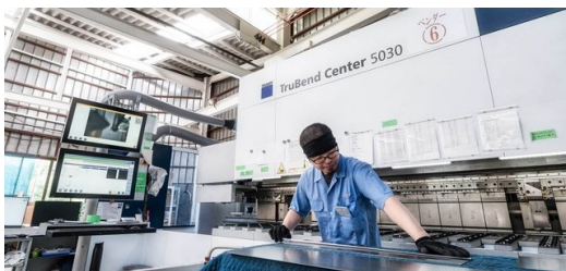
An employee working with the TruBend Center 5030 : This is how the "Orisu" chair is made.
