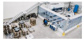
With its 230-tonne press force, the TruBend Cell 5000 can process components of  $3000 \times 1500$  millimeters conveniently.
