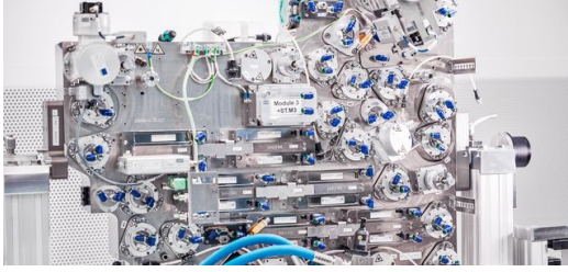
Mirror support on a EUV-module
