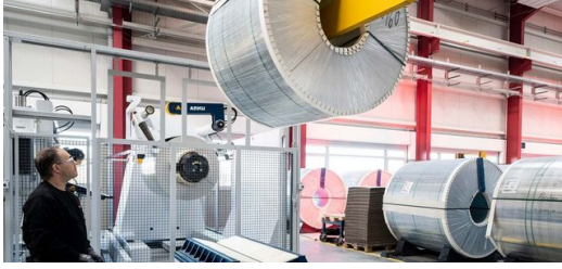
<p>Machine operator Martin Müller heaves a 16-ton aluminum coil into the loading zone of the TRUMPF TruLaser 8000 Coil Edition.</p>
