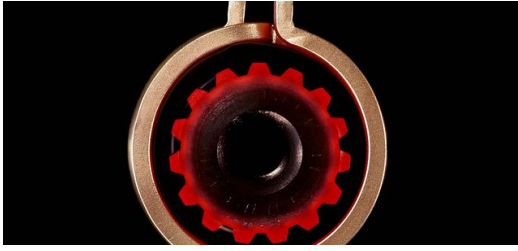
Inductive hardening of a gear part: Like the laser, induction is extremely local. Good conditions for efficient cooperation in flexible process chains. (Image: TRUMPF)
