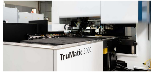
On the TruMatic , hoods shield the processing head, and protective walls on the work table move up if necessary.
