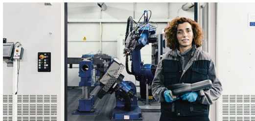
The TruLaser Robot 5020 laser welding system produces very fine and visually appealing seams. This is a key criterion, especially in the furnishings industry with its high share of visible parts. Machine operator Sandra Panedas is very much aware of the benefits this system offers, and Luis Voces praises her skill in using it. (Picture: Niels Schubert)
