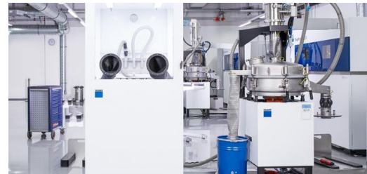
The excess powder is channeled from the unpacking station (left) to the sieving station. This unit cleans the excess powder so that it can be reused. It does this by removing the smoke residue and dirt particles picked up by the powder during the welding process. (© Clauss Morgenstern)
