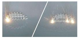
The system operates on the multi-laser principle and is equipped with three scanner-guided and 500-watt TRUMPF fiber lasers.
